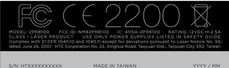
This product contains Class 3B laser, which can produce hazardous level of Class 3B and 4 laser radiations. However, the design of this product incorporates optics, a protective housing and scanning safeguard such that there is no access to level of laser radiation above Class 1. Only trained factory service personnel should open the protective housing.
